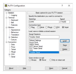
From the 'Serial' menu category, set the serial line COM port, speed 115200 baud, 8 data bits, 1 stop bit, no parity and no flow control.
